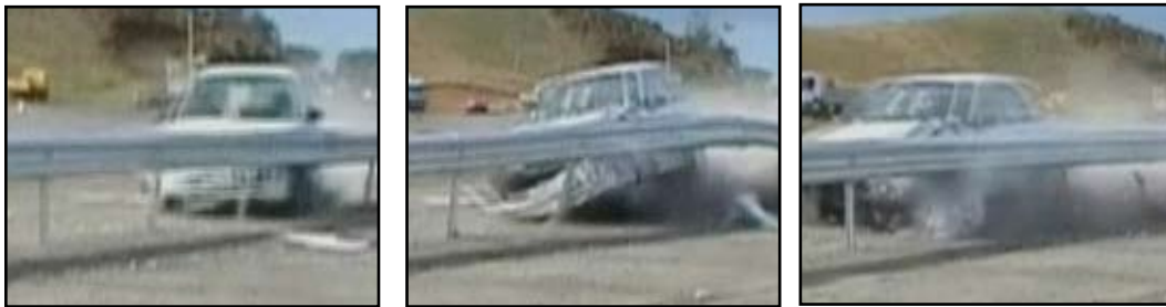
Test Level 3 crash test of NU-GUARD-31 design.
