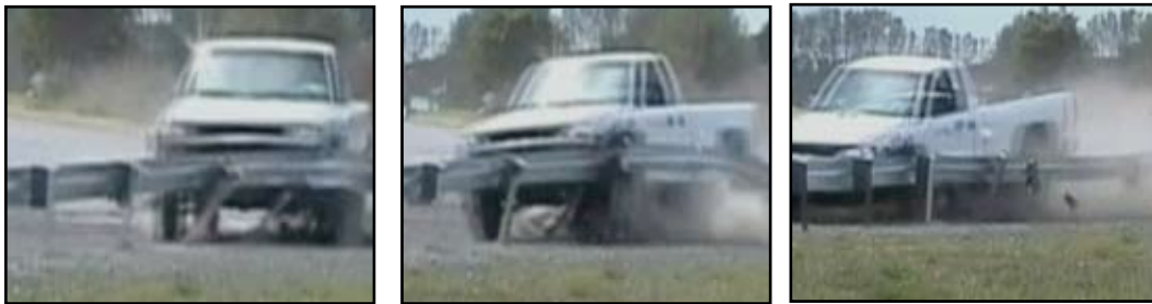
Test Level 3 crash test of NU-GUARD-27 design.
